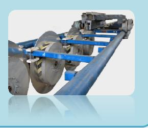
Also, more conductor disks in parallel can push as many magnetic pads, increasing the drive strength and limiting the launch length.
